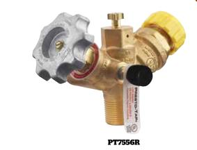
PT7556R version with the service valve closed the pressure test port will be isolated from the container. This will allow a high-pressure leak test to be conducted without disconnecting the pigtail from the service valve.
