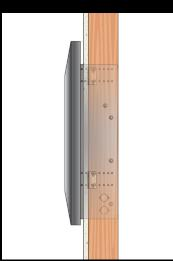
Partially Recessed Installation shown in 2x4 stud walls (Framing: 18" x 30-3/4" x 3-1/2")
