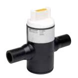
The Elster Perfection PSV polyethylene shut-off valve replaces non-PE and metallic valves to provide economical compatibility with all PE gas distribution systems. These PSV® valves eliminate the need for corrosion inhibiting coatings, cathodic protection, federally mandated corrosion inspection and record-keeping.
