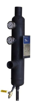
The **FILTAIRE™** is a filtering device designed to trap heavy hydrocarbons commonly present in LP gas vapor and other materials that may be in the gas due to storage conditions and internal conditions of the equipment.
