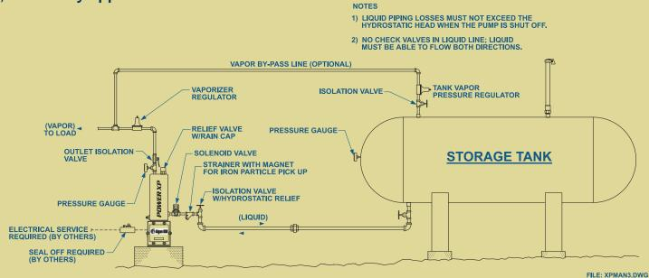
Note: No check valves in liquid line; liquid must be able to flow in both directions.
